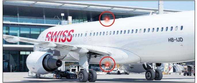
If the red lights (beacons) on the aircraft are flashing, you **may still pass** with great caution. The aircraft could start pushing back at any time.
