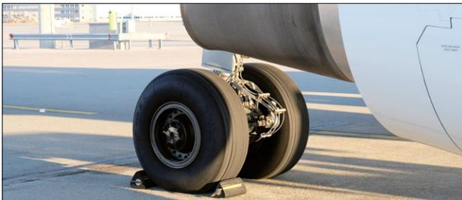
As long as the chocks are still in place, **you may pass the aircraft.** Always watch out behind the aircraft if the engines are switched on.
