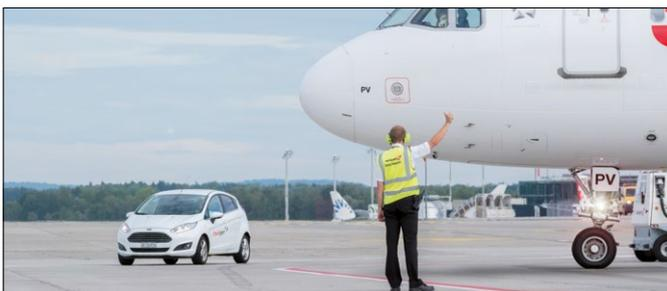
As soon as the chocks are removed, you **must not pass** in front of or behind the aircraft. The "thumbs-up" hand signal is for the pilot.
