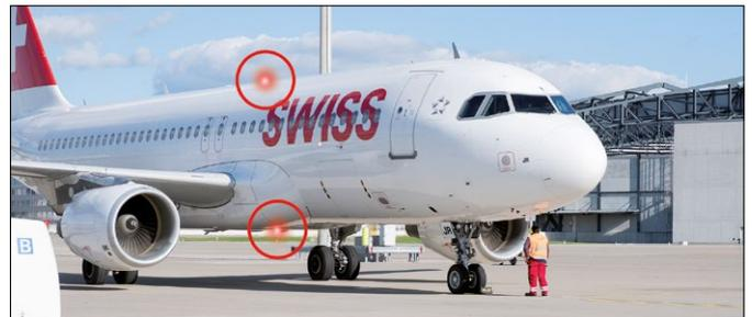
As soon as the red flashing lights (beacons) on the top and bottom of the fuselage are turned on, the chocks may be removed imminently. You may still pass the aircraft **with great caution.**
