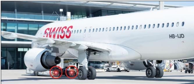
Once the hazard lights on the pushback tractor start flashing, **passing behind the aircraft is forbidden.**
