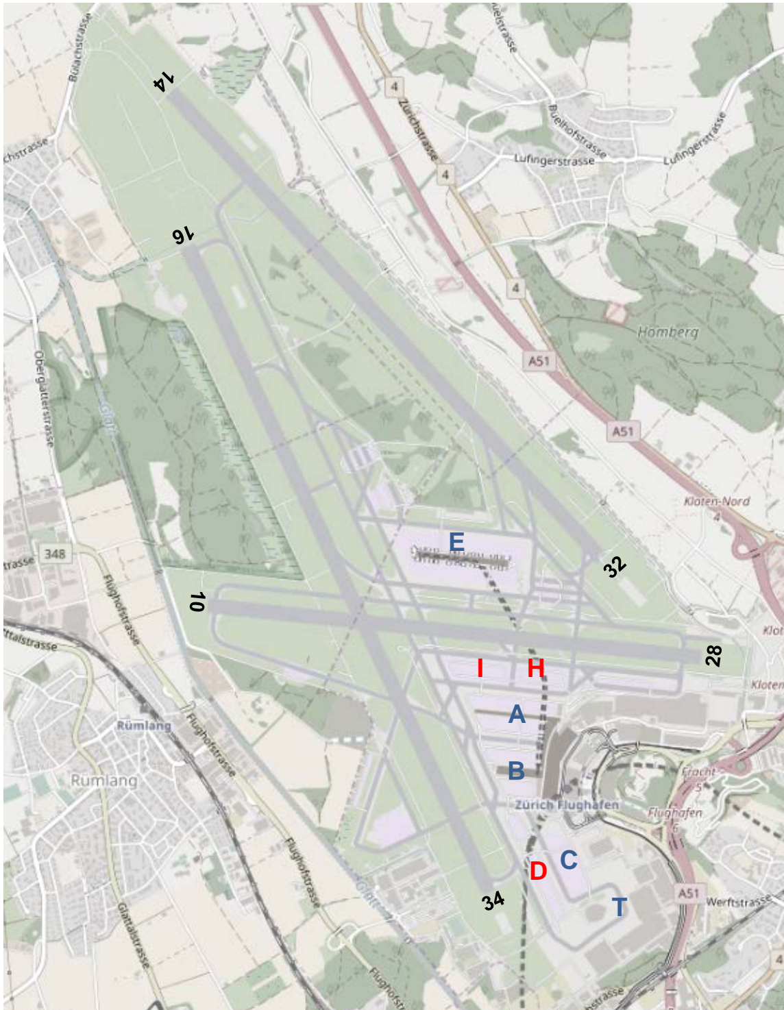
Zurich Airport map with Runways (numbers) and main aircraft stands (blue: push-back; red: self-power)
