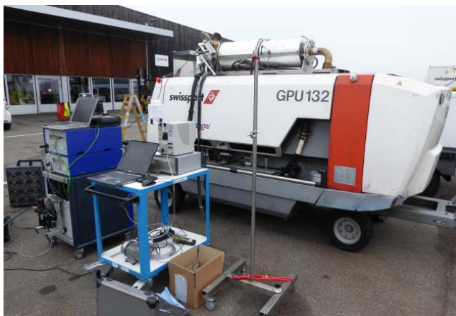
Figure 5 GPU emission measurement set-up
