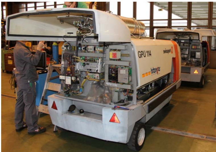
Figure 4 Retrofitting a GPU with a DPF
