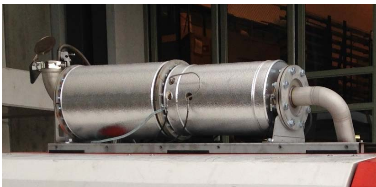
Figure 3 Diesel particle filter (left part) with heating coil (right part), Hug Engineering [2]
