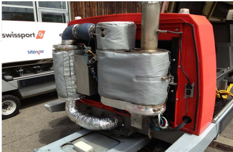
Figure 2 DeNOx and DPF system used for field testing
