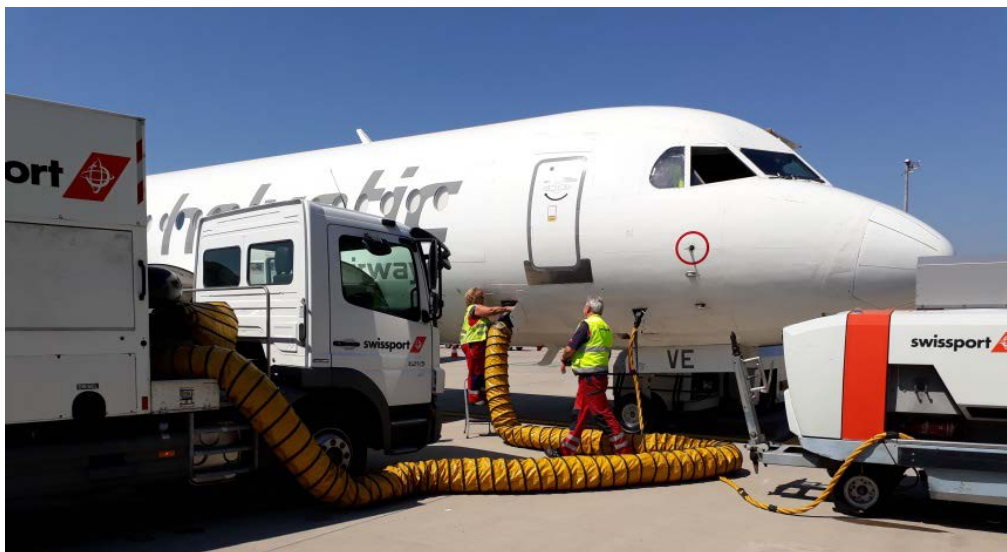
Figure 14 Air Climate Unit (ACU) on the left and Ground Power Unit (GPU) on the right.
